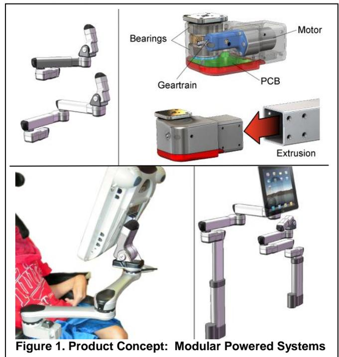
Figure 1. Product Concept: Modular Powered Systems
