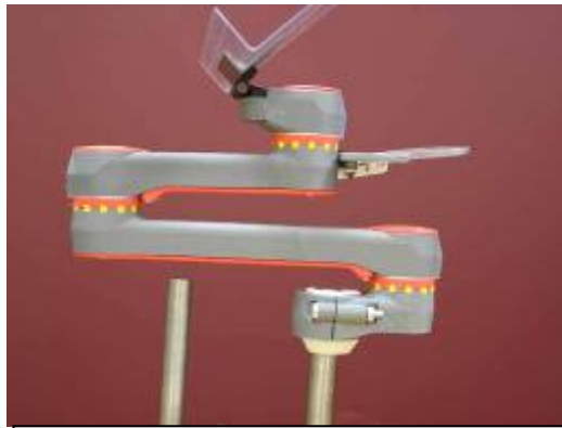
Photo 2. This photograph shows the Double Arm Twistlet Lock Manual Mount used during the usability testing.
