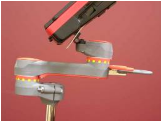
Photo 1. This photograph shows the Single Arm Twistlet Lock Manual Mount used during the usability testing.
