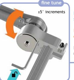
Push tool into slot until the shoulder joint releases
