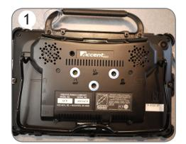
Remove three screws from the back of the Accent 800 or the 1000. Place the nylon washers over the three holes.
