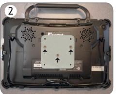
Line up the DP-PRC5 over holes and attach the plate with the three screws that were included with the PRC5 plate (6-32 x 1/2").
