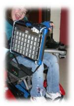
Easily moves out of the visual field for driving (by tilting or rotating device)
