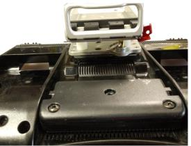
Top view of the quick release plate (QRP) attached to the DP-PRC4 (ring is flipped to the inside)
