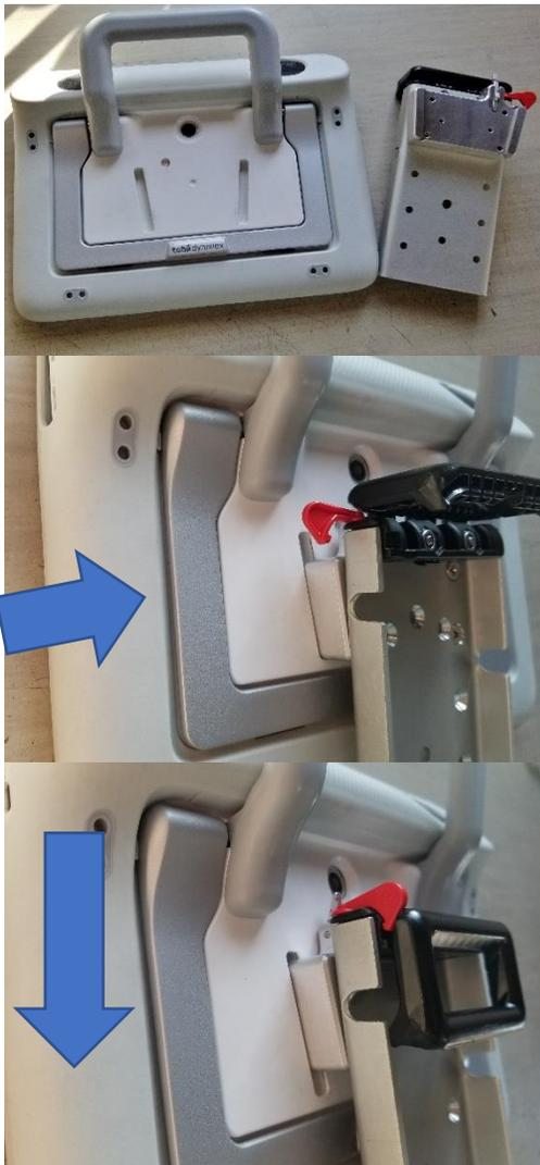
The Indi device (with mounting boot) has integrated mounting slots compatible with the quickconnect
