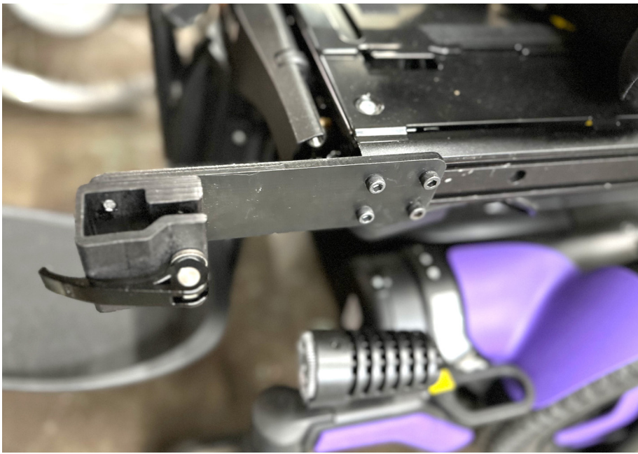
WB2-EXT attached to the Permobil seat rail track
