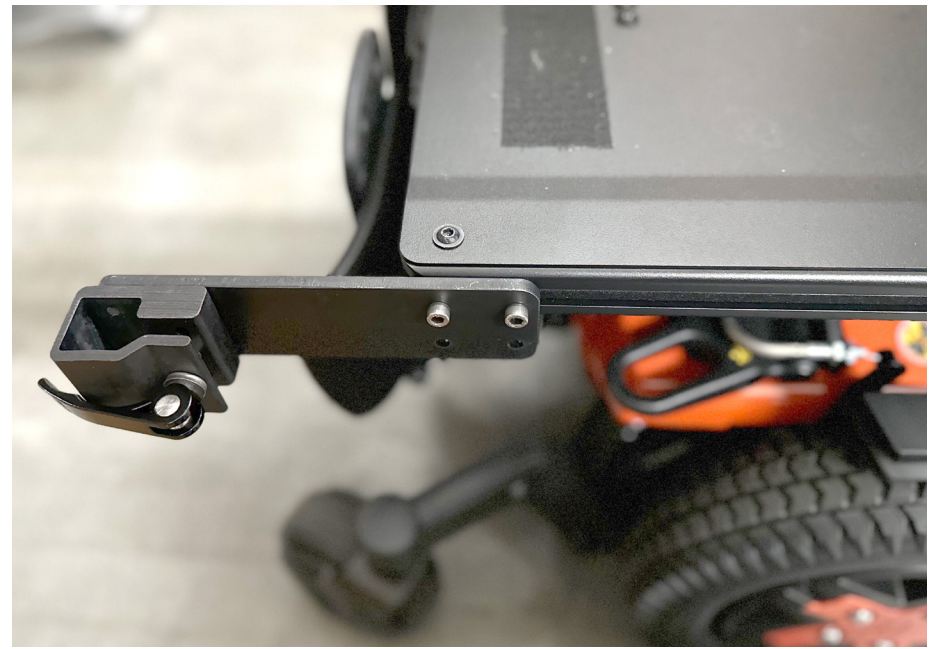
WB2-EXT attached to the Quantum Edge 3 seat rail track...requires a T-Nut
