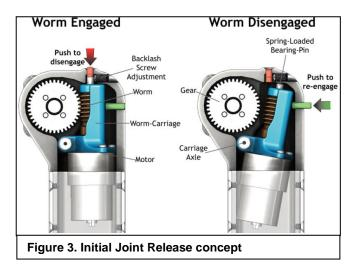
The joint is designed to hold its position without the need for power, minimizing battery draw and allowing it to hold its position when not powered. The gear train incorporates a worm gear, which drives it when the motor is operating, but holds it in position when the motor is not running.
