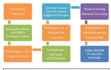
Figure 4. Iterative design process: Joint Release
