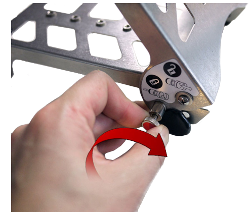
Step 7. Unlatch the red pin so it is in a locked position
