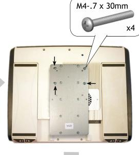
Align device plate over spacers
