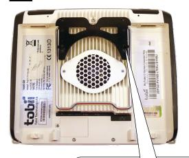
Remove plate and "kickstand" <u>C12</u> on both C8 and C12
