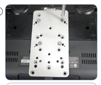
Place DP-PRC1 over the Accent 1400 mounting bracket. Line up the four holes between the two plates and the Accent 1400. Attach using the four screws provided (6/32 x 1/2").
