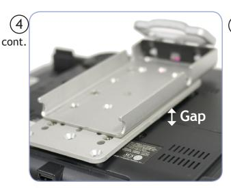
There should be a gap between the DP-PRC1 plate and the Accent 1400 to allow for ventilation.
