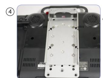
Attach the Quick Release Plate to the DP-PRC1 using the four screws provided (8/32 x 1/4")
